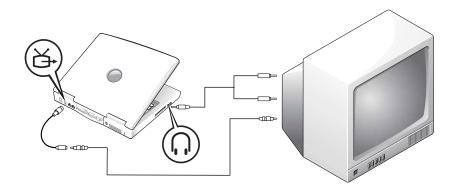
To connect the computer to a television that has a composite video input only, use a composite TV-out adapter cable available from Dell. Before you begin, ensure that you have the following cables:
